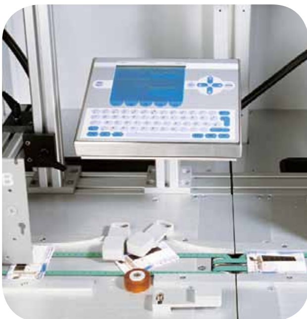
An alphaJET C dual-head unit is incorporated into a Universys from KBA-Metronic, a personalization system for individual cards.
