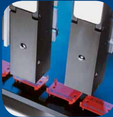
Two networked alphaJET C allow marking with two different colors in one pass.
